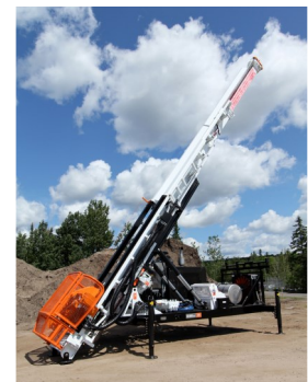
Rotary drilling rig that is being modified for the RAID system.
